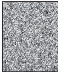
POCO's EDM-C3 is a high quality graphite infiltrated with copper, recommended where speed, wear, and surface finish are important. Unequalled for fragile electrodes, many EDM'ers choose this grade to compensate for operator inexperience or where poor flushing conditions exists.
