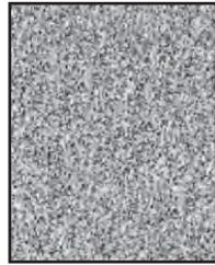
POCO's EDM-AF5 is the premier graphite electrode material available on the market today with an average particle size of less than one micron. This particle structure gives EDM-AF5 superior strength, provides for fine surface finish ( $7\mu\text{inR}_a$ ), gives excellent metal removal rate, and high resistance to wear.
