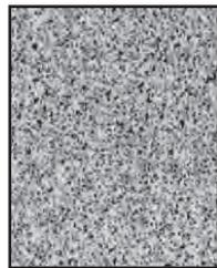
POCO's EDM-3 is an isotropic Ultrafine grain graphite which offers high strength with outstanding wear and fine surface finish characteristics easily machined to thicknesses of 0.1mm or less.
